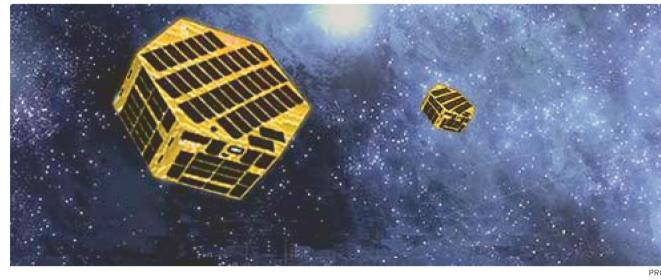
**Above:** The CUSat team's Web page logo shows an artist's conception of the satellite after it has separated in orbit. **Right:** One half of the CUSat satellite. In orbit, two identical halves will separate to test tracking and imaging software.
